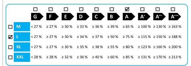
Water heating energy efficiency under colder and warmer climate conditions
